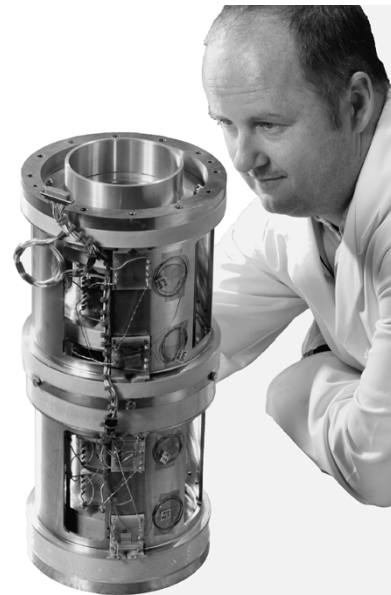
Fig. 6. Completed ADR magnet system, after testing.
